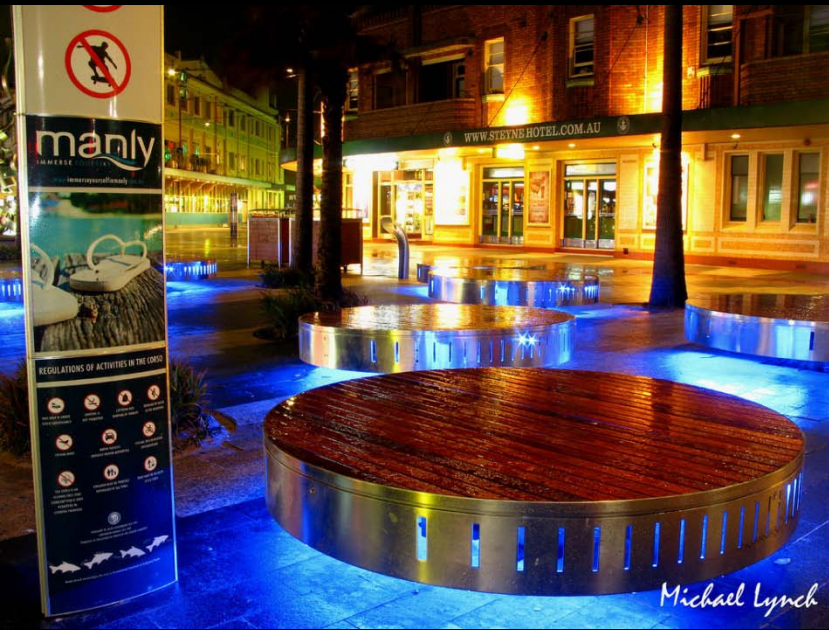
“SOFA – Timber platforms with laser cut steel bases, highlighting perforations and the base of seating elements”
