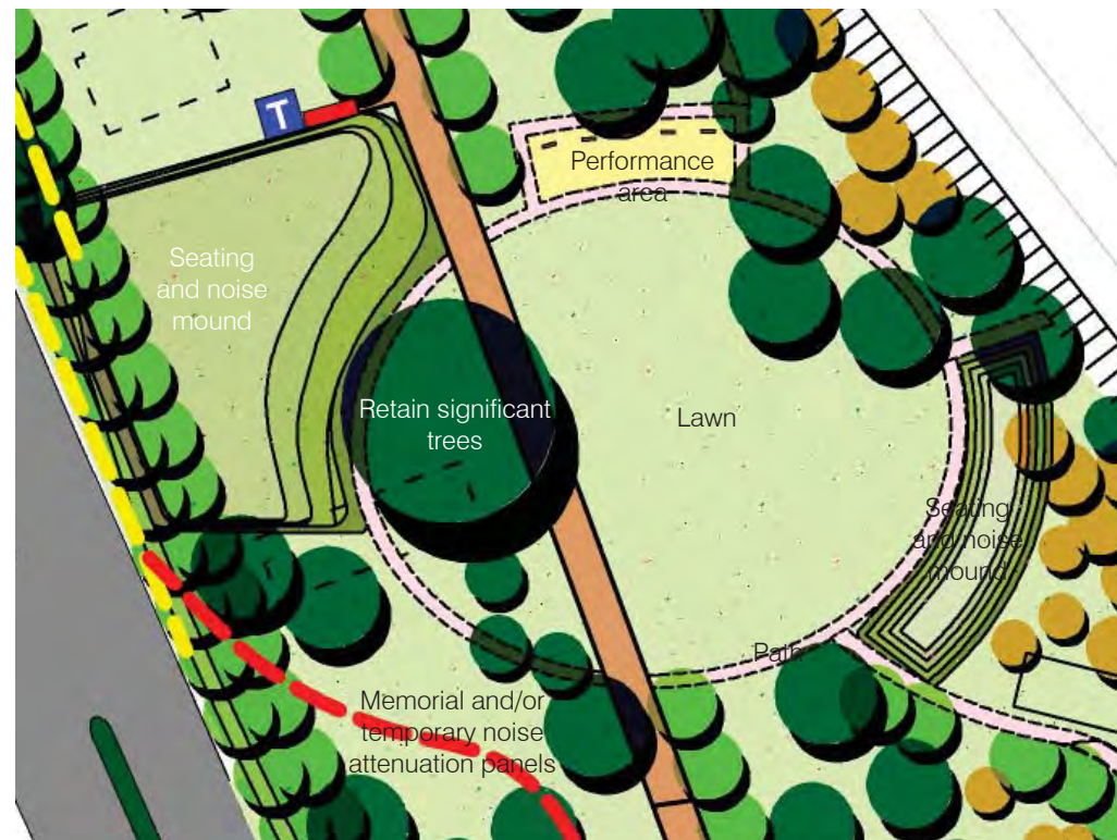
Sound Garden incorporates existing significant trees, seating and sound mound along Princes Highway, a rounded open grassed space for events and a smaller formal zone to the north, which functions as the base for a temporary stage. This stage is placed at an angle to reduce sun glare to performers and direct sound south, away from residents to the east.
