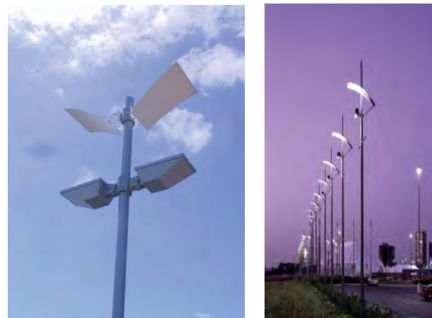
Narrow, tall pole lights with reflective shields.
